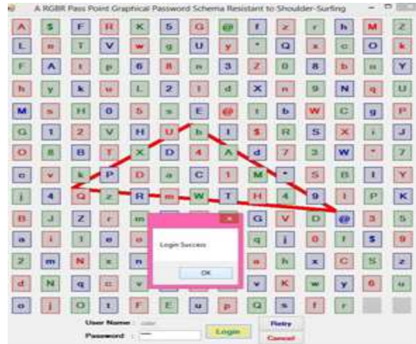
Figure 17: Triangle Formed by Clicking on the Cells “Qb@b” Containing the Color Red, Green, Blue and Red Respectively for Login Attempt
