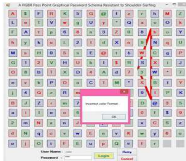
Figure 18: Triangle Formed by Clicking on the Cells “3@b3” Containing the Green, Blue, Red, and Green Respectively for Login Attempt. Incorrect Color Format
