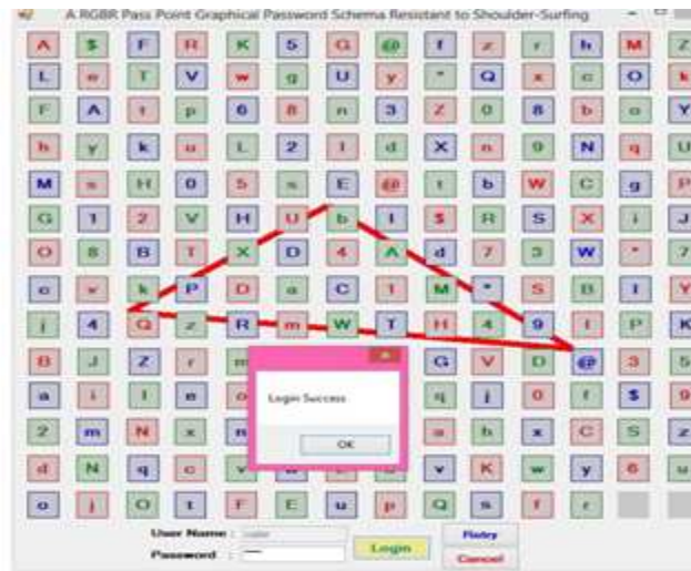
Figure 12: Triangle Formed by Clicking on the Cells “Qb@Q” Containing the Color Red, Green, Blue and Red Respectively for First Login Attempt
