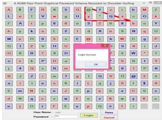
Figure 14: Triangle Formed by Clicking on the Cells “b@3b” Containing the Color Red, Green, Blue and Red Respectively for Second Login Attempt
