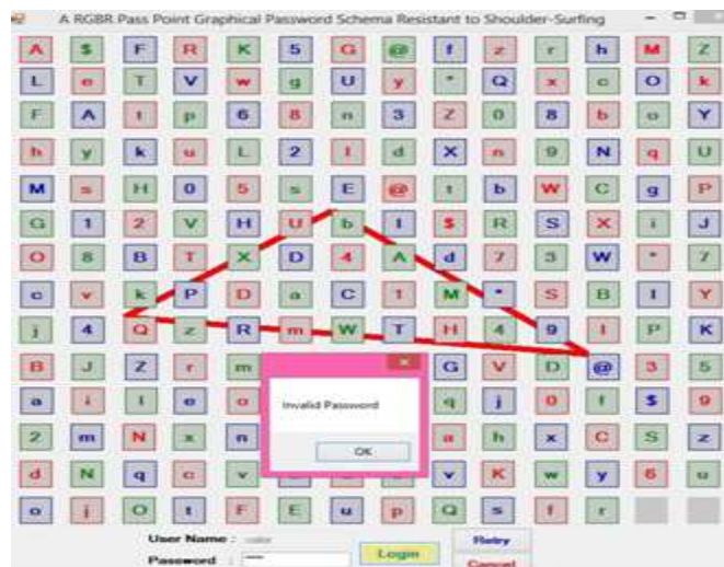
Figure 13: Triangle Formed by Clicking on the Cells “Qb@Q” Containing the Color Red, Green, Blue and Red Respectively for First Login Attempt Repeated Successively. Login Failed
